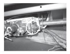
Locate the ground lug at the receptical box, left of the unit.
